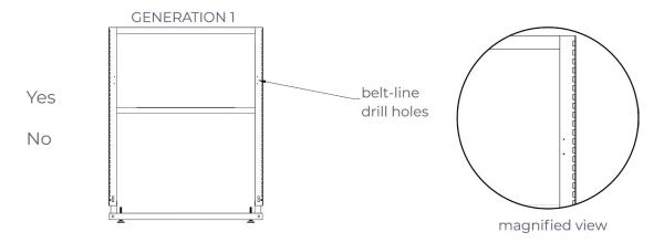
Does the Cosmopolitan panel frame have drill holes on the front face as shown in the picture below?
