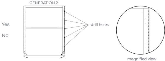
Does the Cosmopolitan panel frame have square and drill holes on the front face as shown in the picture below?
