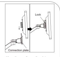
Hang the monitor on the plate from top to bottom and ensure it be tightened
