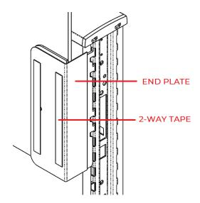
3. Align the fascia edge with the glass panel edge. Press the fascia onto the twoway tape on the end caps.
