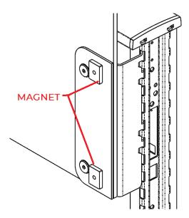
2. Align the fascia with the glass panel edges. Attach fascia to the magnets.
