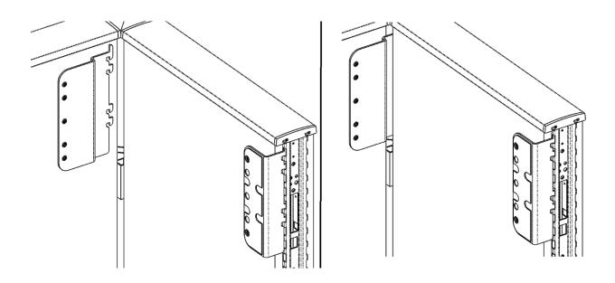
3. Attach the L-bracket aligning to the countersink holes on the middle three holes on the Z-bracket.
