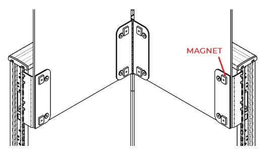
2. Align the fascia with the glass panel edges. Attach fascia to the magnets.
