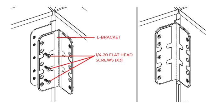
4. Install the glass, or laminate panel by aligning the holes on the panel to the holes on the end brackets. Attach the  $\frac{1}{4}$ "-20 screws through the holes and onto the end brackets and Z/L bracket assembly.
